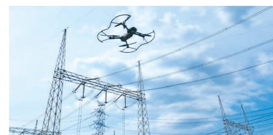
Drones (left) and small camera-equipped robots (right) are being considered for investigating the insides of substations.
